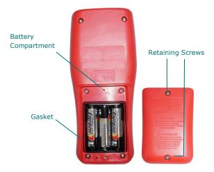
Figure 1: Battery Installation
