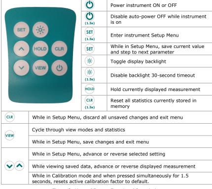
Figure 2: Keypad Button Functional Description
