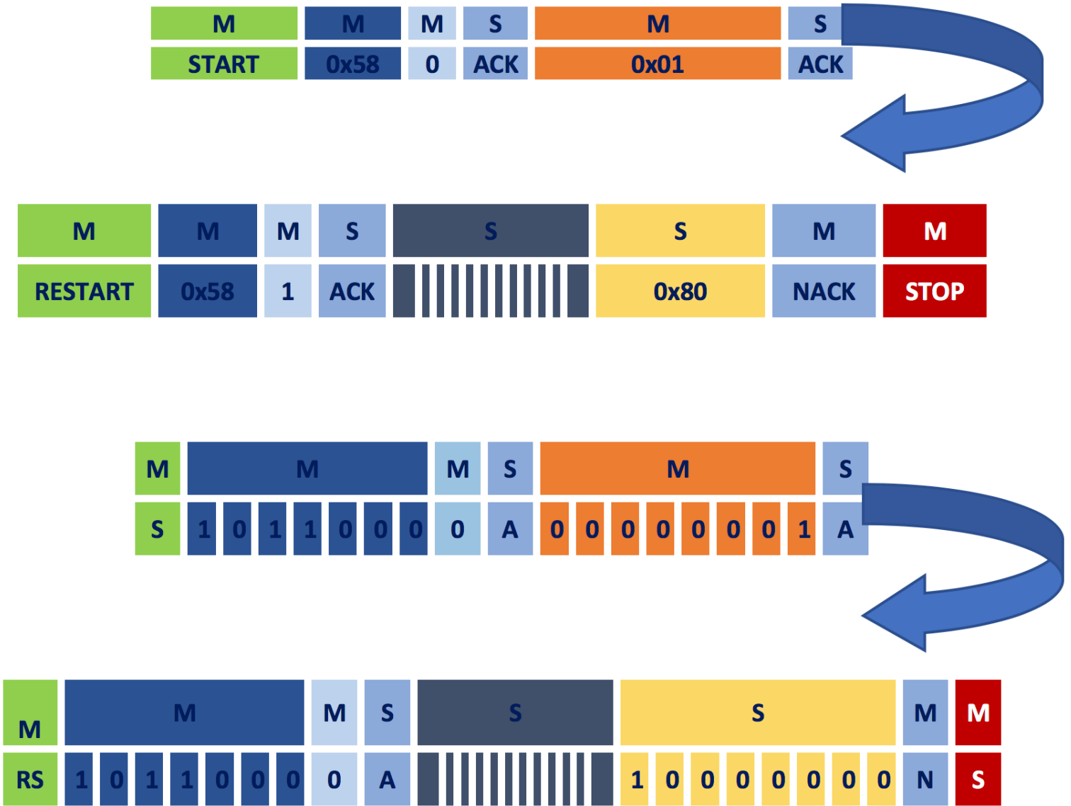
Figure 19: Example to read last control command
