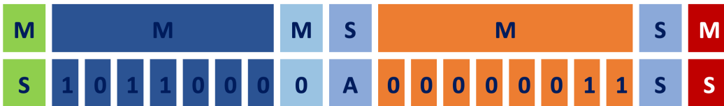
Figure 7: Example for I 2 C Command 0x03 "Clear all Faults"
